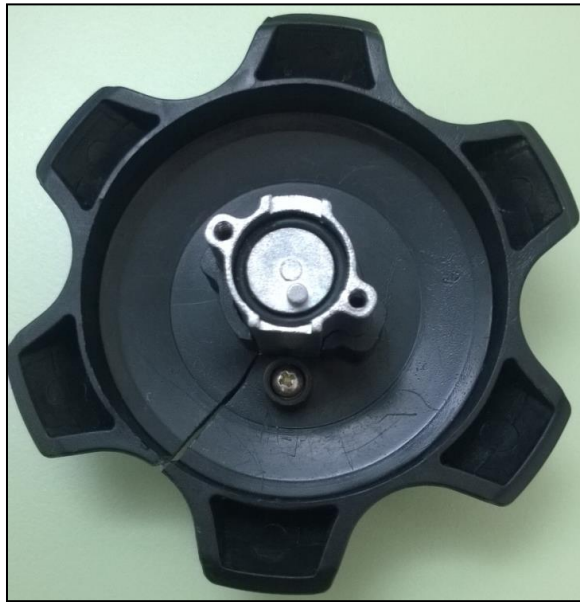
Figure 1. Failure in fuel cap
